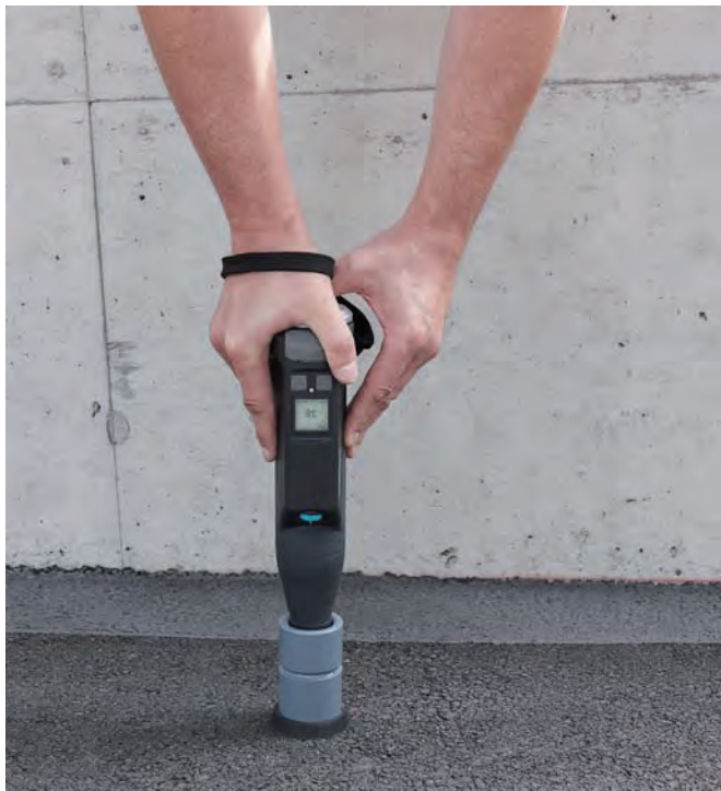
Original Schmidt Live with portable testing anvil
